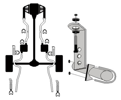
Hanger consists of a metal strap, grommets, hardware and clamp (see illustration).
