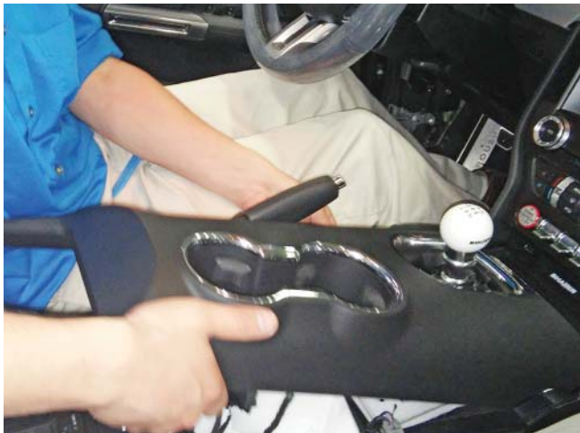
27. With the emergency brake fully engaged, lift the top portion of the center console up and unplug the connectors for the key fob detection circuit and for the cup holder lighting (if equipped). Pull back on the center console to release the clips.
