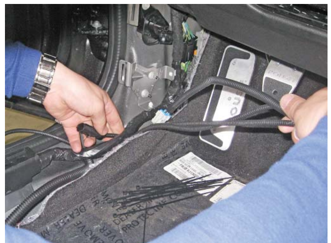
29. Continue routing the wire harness up through the driver side kick panel area and secure as shown below.
