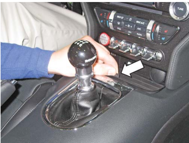
26. Using a non-marring trim tool, gently lift each of the rear corners of the center console and disengage the retaining clips along the bottom from the rear all the way up to the front.
