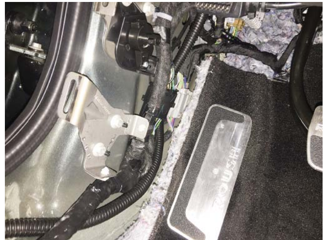
30. Plug the OBDII pass-through connector that is part of the active exhaust wiring harness (P/N: 1315-9L430) into the OBDII connector that is under the dash. Secure the connector with two (2) standard 7" zip ties (P/N: CTUV740) as shown below.
