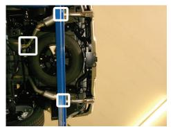
5. Loosen clamp securing muffler to inlet pipe, dismount muffler from factory isolators (x2), unclip ground wire and remove assembly from vehicle.
