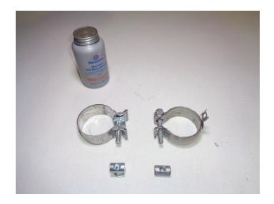
8. Place **clamp (9)** onto **inlet pipe (1)** then connect it to factory pipe; line up inlet pipe notch with factory pipe tab then slide them together. Tighten clamp just enough to allow for adjustment.
