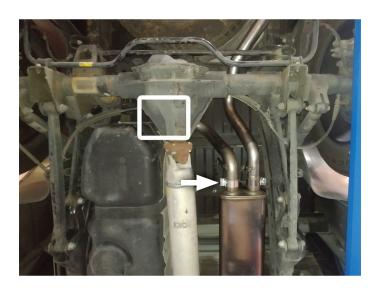
12. Place clamp (8) onto left rear tailpipe (5), connect it to left front tailpipe and insert wire hanger in isolator. Tighten clamp just enough to allow for adjustment.
