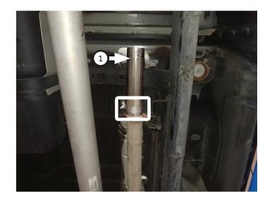
9. Place clamp (9) onto muffler (2) inlet then connect it to inlet pipe. Tighten clamp just enough to allow for adjustment. Place (x2) clamps (8) onto muffler outlets.
