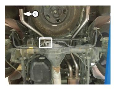
13. Place (x2 ea.) clamps (8) onto exit pipes (6) then connect them to tailpipes. Tighten clamps just enough to allow for adjustment.
