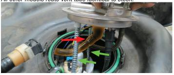
**NOTE:** If the factory fuel tank pressure sensor connector does not fit onto the new fuel tank pressure sensor, remove the sensor from the old fuel pump and install it onto the new fuel pump.
