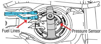
12. Install a J 45722 fuel pump lock ring tool or equivalent to the pump's lock ring.
