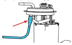
16. Remove and discard the fuel pump 0-ring seal as a new one is provided in this kit.
