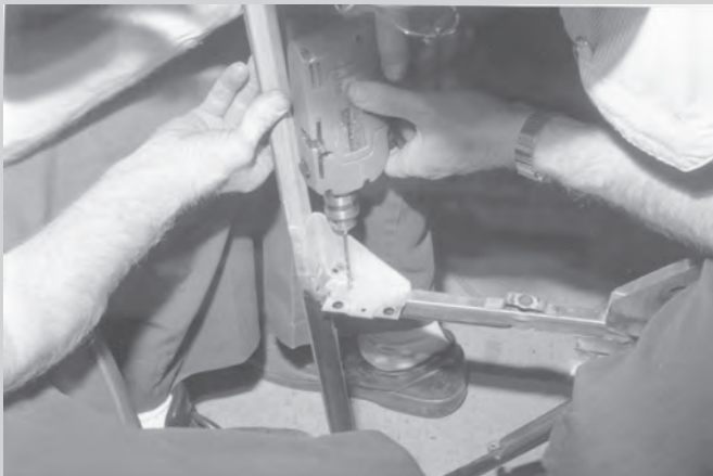
With electric drill, remove rivets fastening the old vent window rubber seal to the top and the bottom of the frame.
