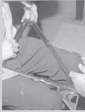
Install new vent window rubber seal using silicone spray and small screw driver. Be sure to set firmly in grooves.
