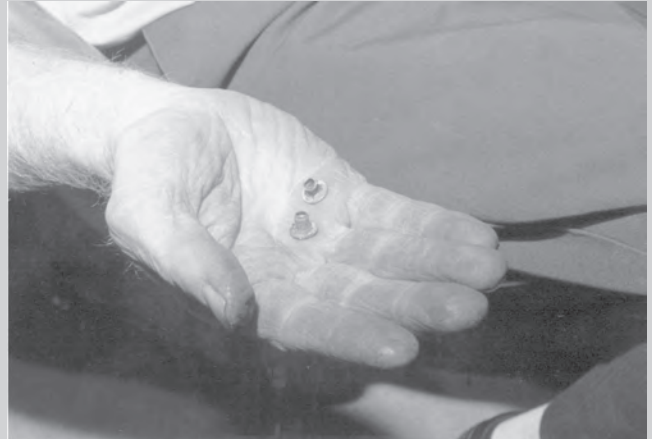
IMPORTANT! When drilling out rivets, save rivet sleeves for reuse.
