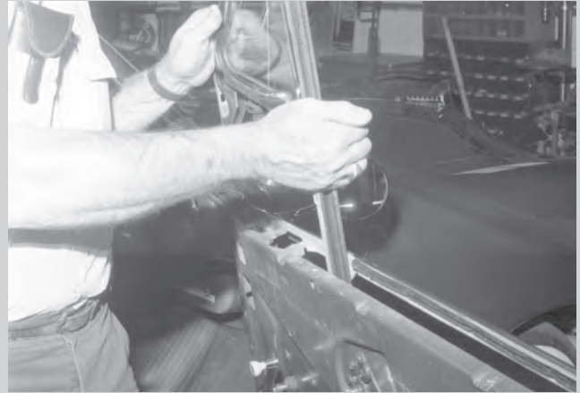
Slowly remove division bar and vent window assembly from the door.
